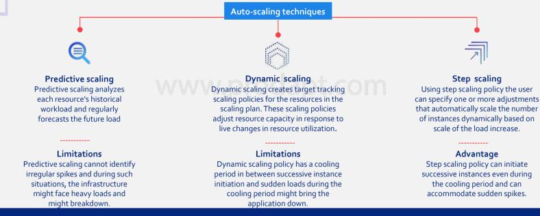
The agility of the infrastructure provisioned mainly depends on the strength of scaling policy defined. Step scaling policy is the most recommended technique to handle peak irregular loads.
