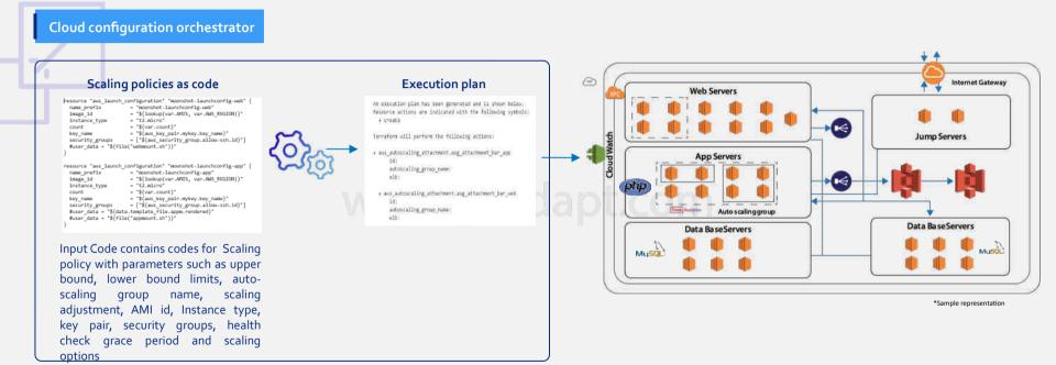
\*The scaling policies from the orchestrator gets integrated with monitoring tool (Amazon cloud watch). It dynamically monitors the entire infrastructure and triggers the scaling mechanism on reaching the threshold.
